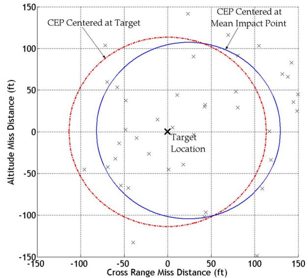
**Fig. 3 Uncontrolled dispersion (CEP=113.5 ft centered at mean impact point)**
