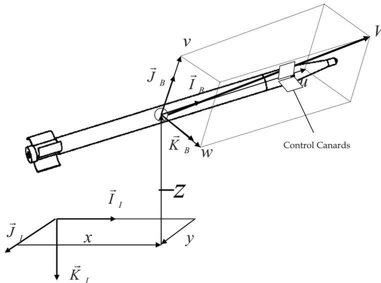
Fig. 1 Schematic of the position coordinates of a direct fire projectile
