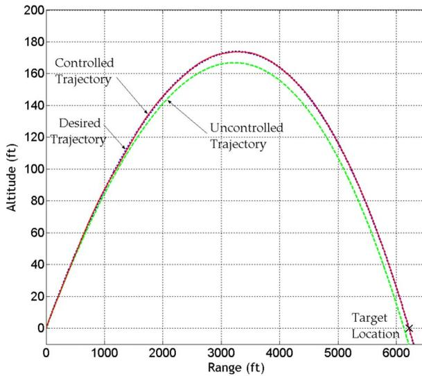
Fig. 5 Typical altitude versus range
