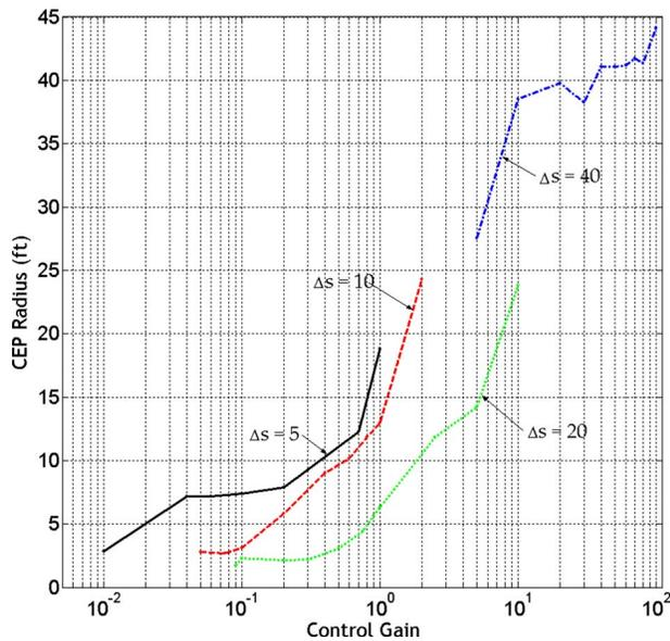
**Fig. 12 Controlled dispersion results as the arc length step size is varied**
