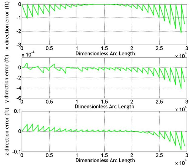
Fig. 7 Error between linear and nonlinear trajectory solutions
