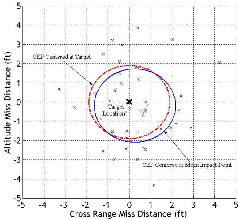
Fig. 9 Controlled dispersion with sensor bias and noise applied (CEP =2.1 ft centered at mean impact point)
