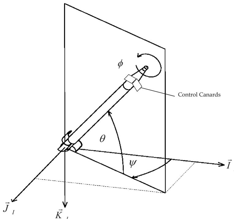
Fig. 2 Schematic of the attitude coordinates of a direct fire projectile
