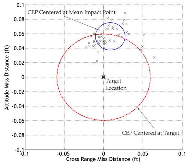
**Fig. 4 Controlled dispersion (CEP=0.02 ft centered at mean impact point)**
