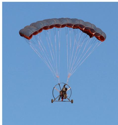
**Fig. 4 Small-scale parafoil and payload system used for experimental flight testing**
