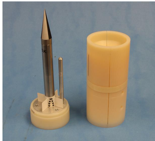
Fig. 13 Fully integrated active projectile and sabot assembly
