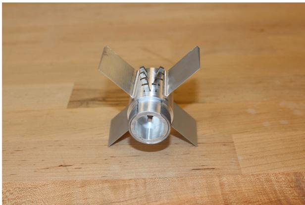
Fig. 12 Fully assembled active microspoiler assembly in aft section of projectile
